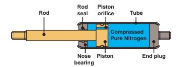
A gas spring is basically a system consisting of a pressure tube, rod and piston. The energy for the spring is provided by gas at high pressure and the whole system is self contained and sealed against loss.
